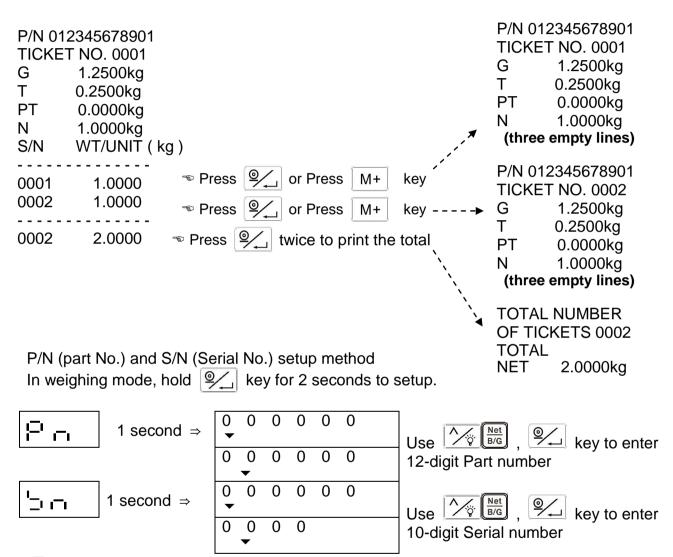
After power-off, S/N will reset as 1. P/N will be saved in memory, available during next power-on.
