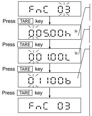
LCD displays the last saved status. Key in the desired high limit value, then press TARE key.
