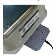
Try to move around the charging plate and ensure it is unmovable
