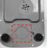
Raise the scale and aim the point near the center. Slide the charging pad and attach to the position hole
