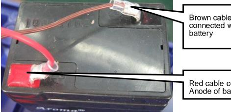
Brown cable(or black cable) connected with Cathode of battery
